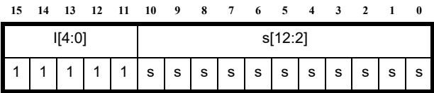
Figure 9-25 Compact Branch and Link Unconditionally Format
