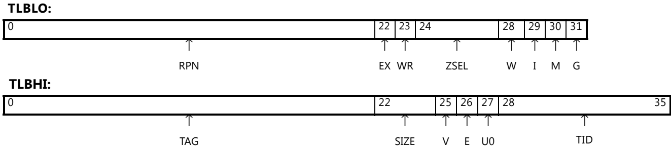
Figure 2-20: TLB Entry Format
