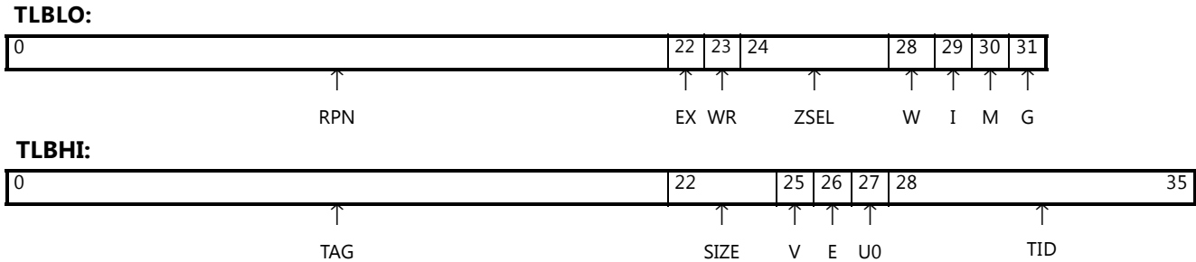
Figure 2-20: TLB Entry Format
