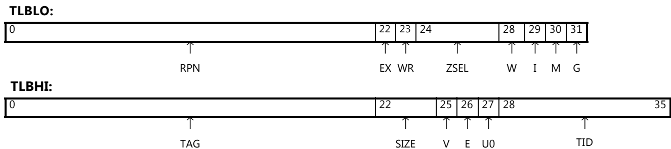
Figure 2-20: TLB Entry Format (PAE disabled)
