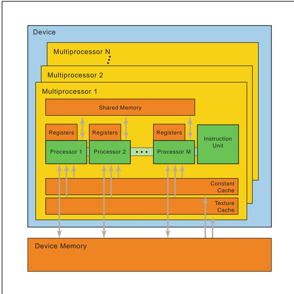
A set of SIMT multiprocessors with on-chip shared memory.
