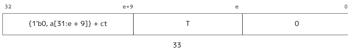
Figure 16. Decoding of the XLEN+1 wide top (t) bound
