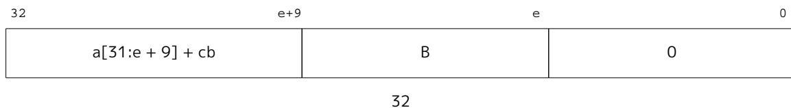
Figure 17. Decoding of the XLEN wide base ( b ) bound
