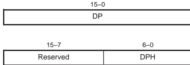
The CPU can concatenate the two to form an extended DP that is called XDP (see Figure 2–8 and Table 2–7). The high part (DPH) is used to specify the 7-bit main data page for accesses to data space. The low part specifies a 16-bit offset (local data page) that is concatenated with the main data page to form a 23-bit address.
