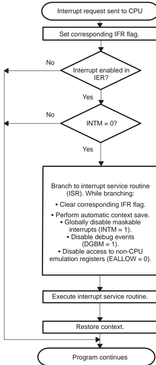
Table 5–3. Steps in the Standard Process Flow for Maskable Interrupts
