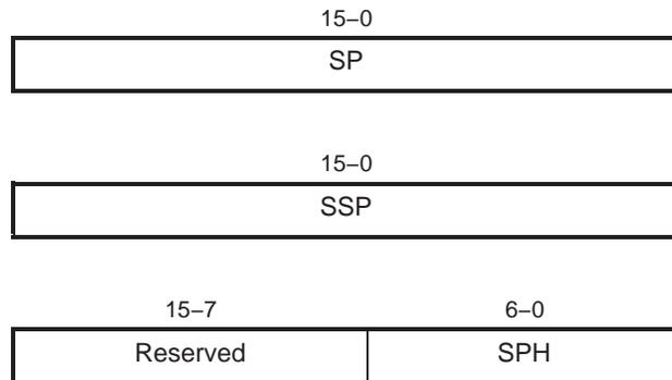
See Figure 2-10 and Table 2-8. When accessing the data stack, the CPU concatenates SPH with SP to form an extended SP that is called XSP. XSP contains the address of the value last pushed onto the data stack. SPH holds the 7-bit main data page of memory, and SP points to the specific word on that page.
