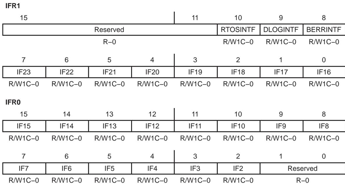
**Legend:** R = Read access; W1C = Writing a 1 to this bit causes the CPU to clear this bit to 0; -n = Value after DSP hardware reset; Reserved = A write to this bit has no effect, and the bits in this field always appear as 0s during read operations.
