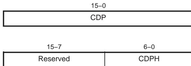
The CPU can concatenate the two to form an extended CDP that is called XCDP (see Figure 2-5 and Table 2-4). The high part (CDPH) is used to specify the 7-bit main data page for accesses to data space. The low part (CDP) can be used as:
