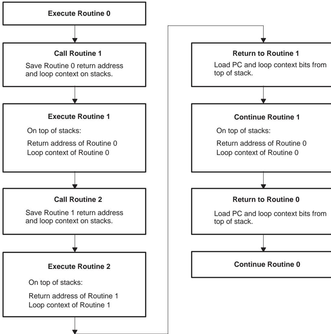
Figure 4-3. Use of RETA and CFCT in Fast-Return Process
