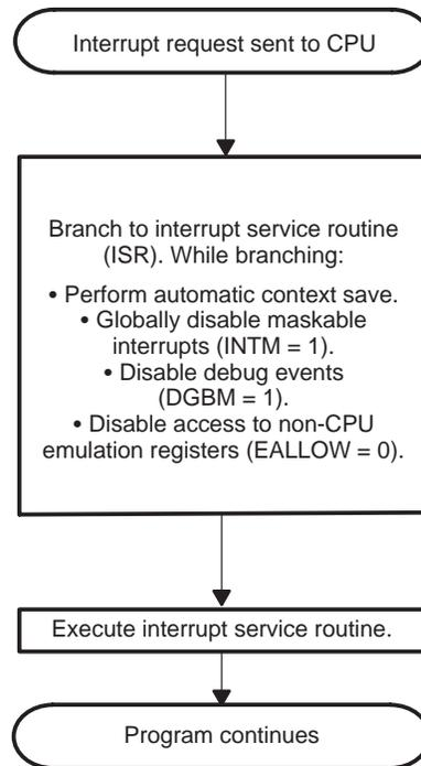
*Table 5–5. Steps in the Standard Process Flow for Nonmaskable Interrupts*
