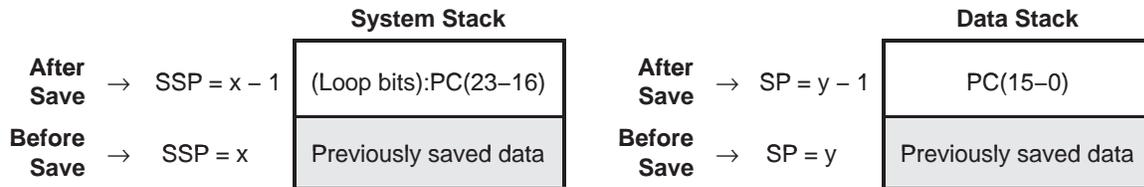
A return instruction at the end of a subroutine forces the CPU to restore the return address and the loop context from the stack. For each stack, the CPU increments the stack pointer (SSP or SP) by 1 after the read from the stack.
