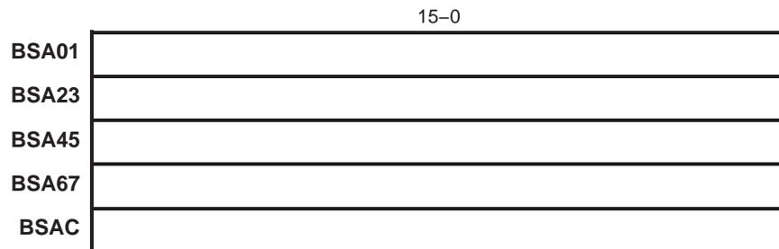
Each buffer start address register is associated with a particular pointer or pointers (see Table 2–5). A buffer start address is only added to the pointer value when the pointer is configured for circular addressing in status register ST2\_55.
